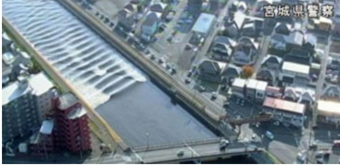
Figure 7: Standing tsunami bore wave in Sunaoshi River, Miyagi Prefecture, Japan 2016. (Miyagi Prefectural Police / Kyodo / Reuters)
